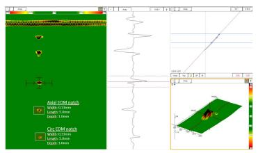
Figure 1: Calibration Tube Scan
