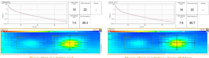
51mm (2in) insulation and aluminum weather jacket
