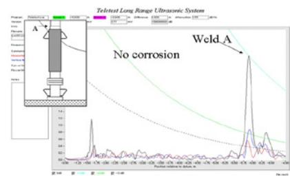
**FOCUS+ scan showing no corrosion**
