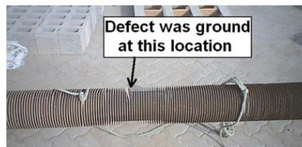
FOCUS+ uses the MultiMode™ system, which enabled inspecting this finned tube using torsional and longitudinal wave modes. Torsional and longitudinal wave modes were found to be affected very differently by the geometry of pipes.
