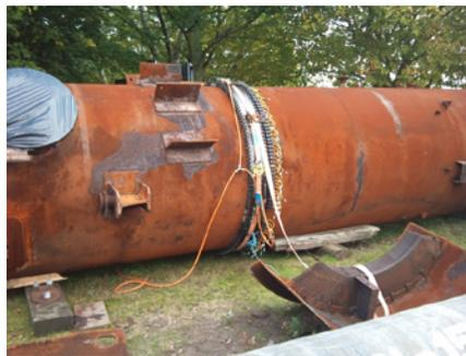
Figure 1. Teletest Focus guided wave ultrasonic test equipment applied to inspect the 66" vessel
