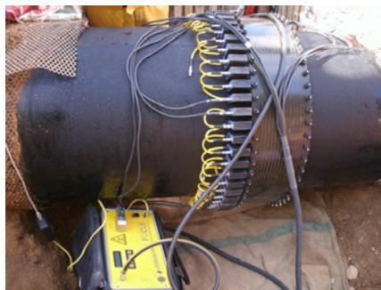
FOCUS+ used to inspect the 61 cm (24 in) buried pipeline through HDPE coating
