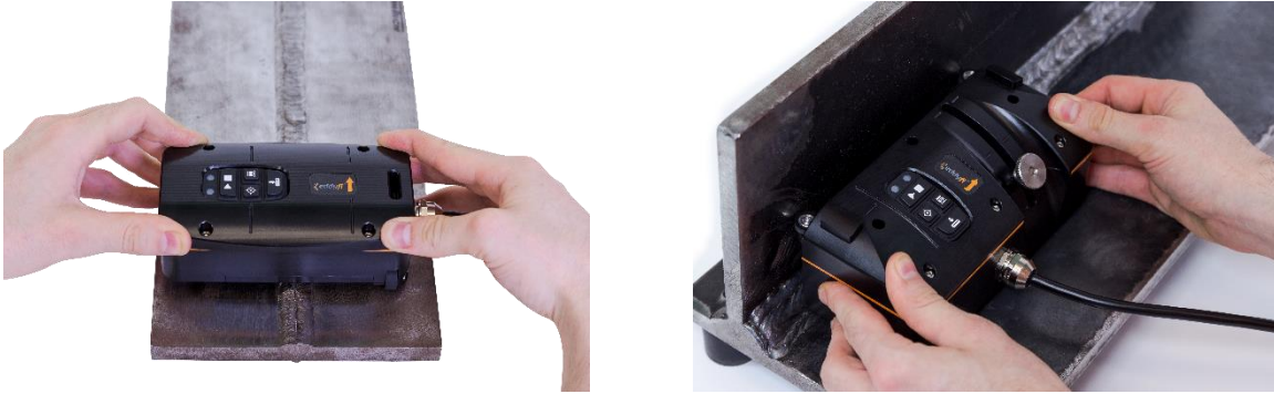
Figure 6. Sharck probes on carbon steel weld
