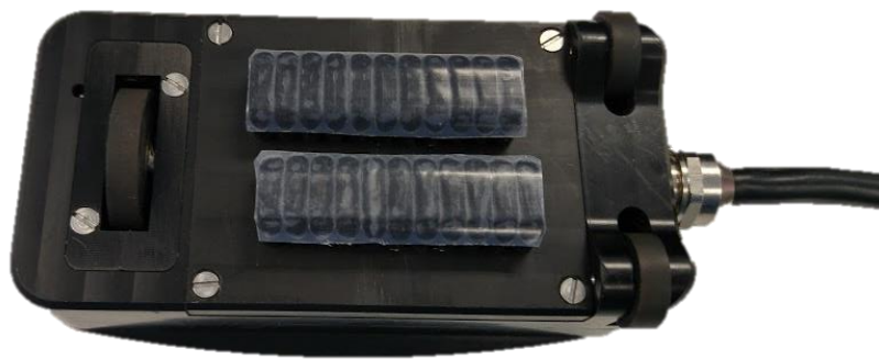
Figure 26. Protective tape applied on probe active area
