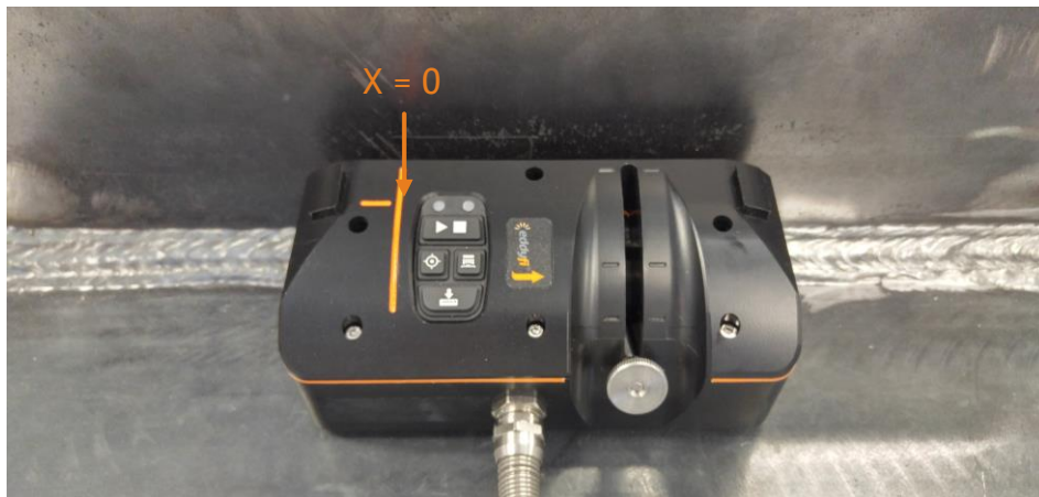
Figure 10. Scan position X=0 aligned with the marker line on the fillet weld probe
