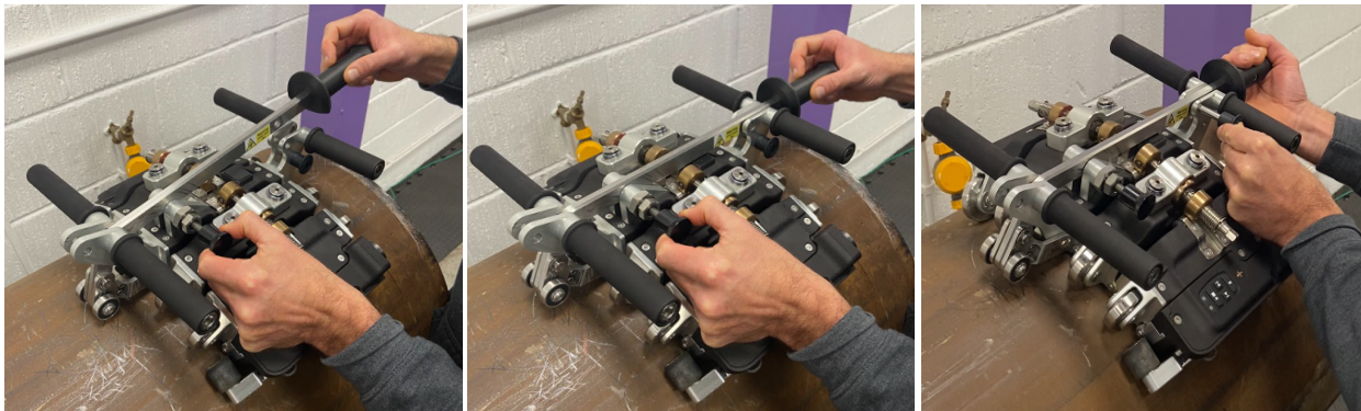
Figure 26: Pipescan HD Deployment 06
