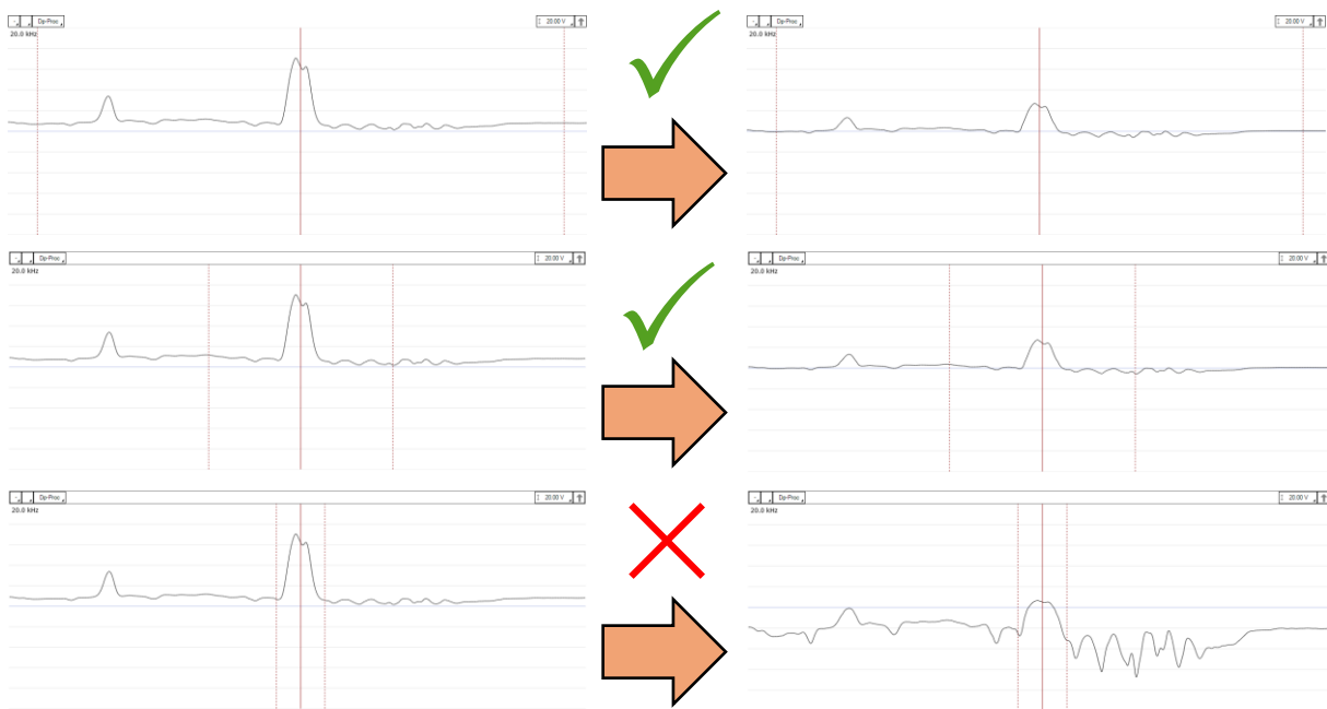
Figure 39 : Top : Good user material calibration, with the C-scan cursor widely opened; Middle : Good user material calibration, cursor contains only one specific crack, but opened wide enough (at least three times the length of the crack) providing a local averaging; Bottom : Bad user material calibration, cursor too closed around the crack signal.
