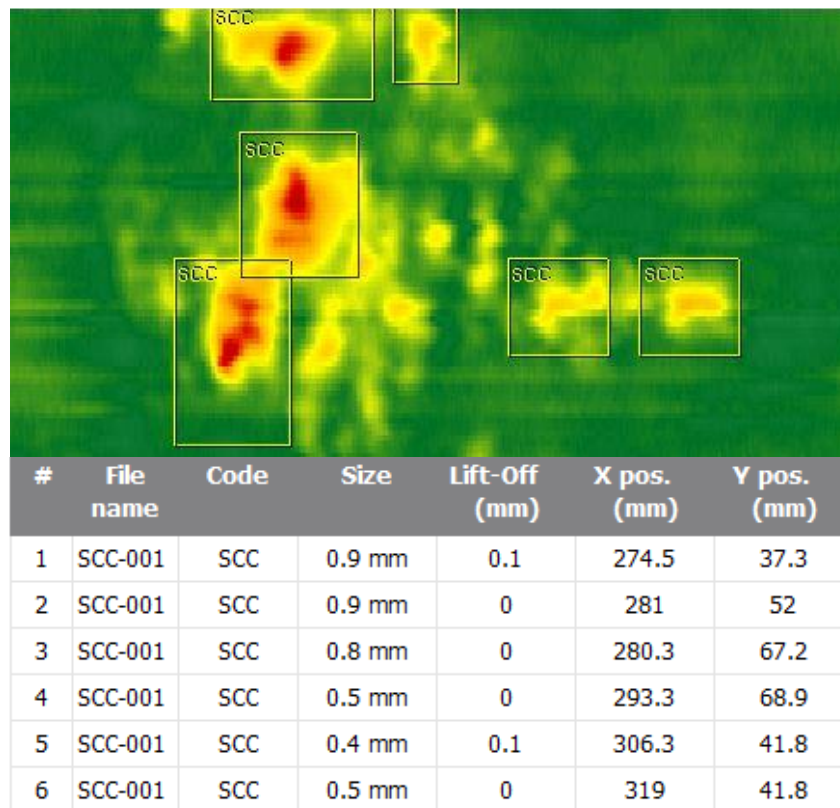
Figure 60. Summary table displayed on the first page of the report, containing information about all the defects that were reported in the current inspection. This is usually followed by individual screenshots and information of all the reported defects.
