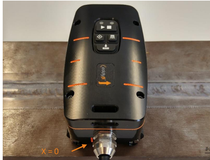
Figure 8. Scan position x=0 aligned with the marker line on the probe side
