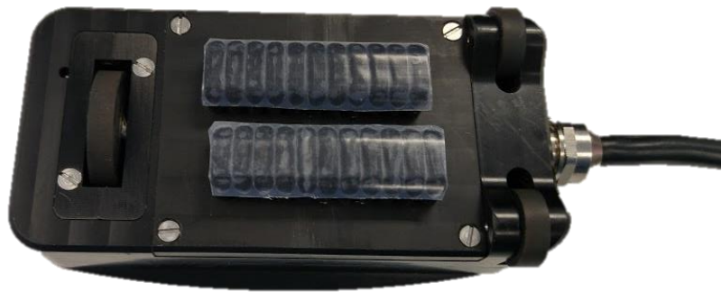
Figure 27. Protective tape applied on probe active area
