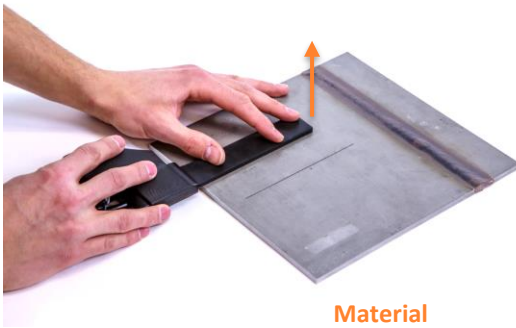
Performing a lift-off with the I-flex probe
