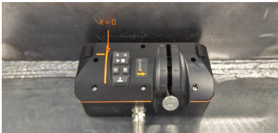
Figure 11. Scan position X=0 aligned with the marker line on the fillet weld probe
