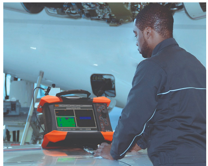
Figure 4: Gekko performs aerospace composite material inspection.
