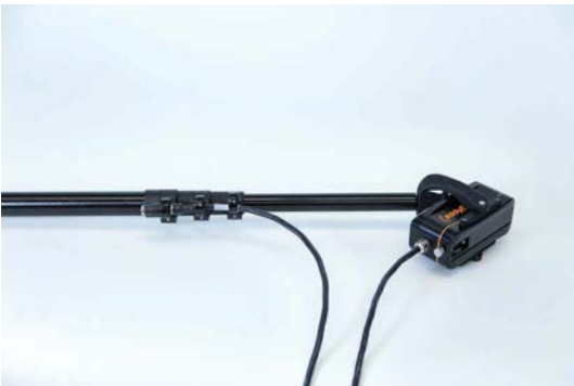
Figure C-5 Running PEC probe cable through pole hoops
