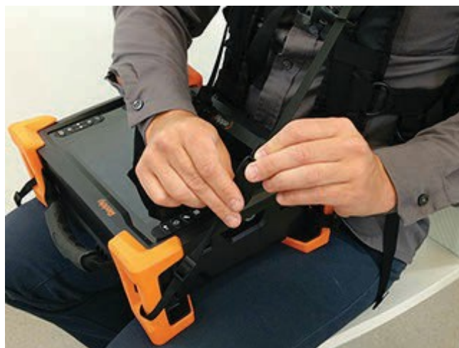
Figure B-15 Mating shoulder anchor strap
