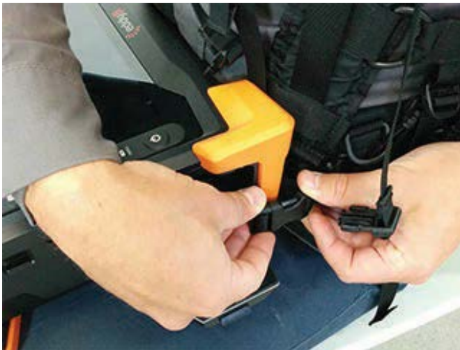
Figure B-13 Mating battery compartment side anchor strap
