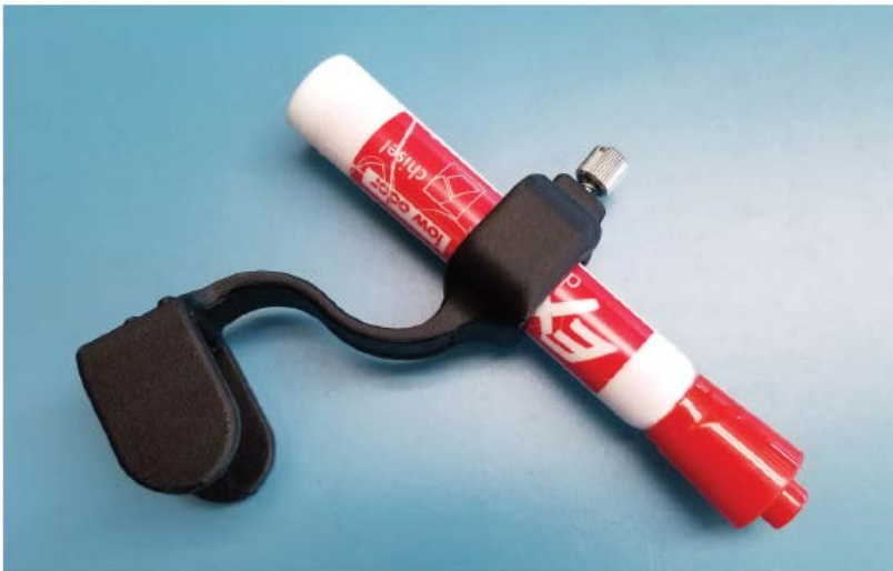
Figure D-7 Erasable marker installed
