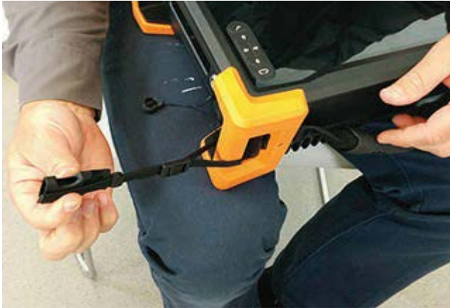
Figure B-10 Alternative method of securing anchor strap to bumper
