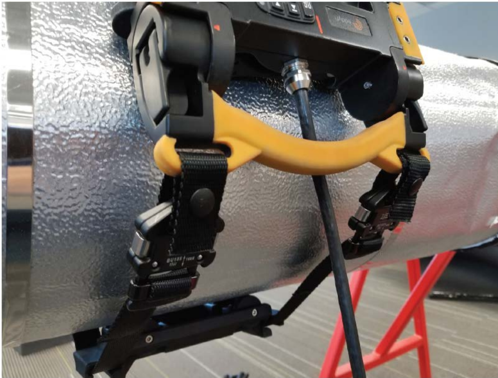
Figure D-5 Strap connected to the probe buckles
