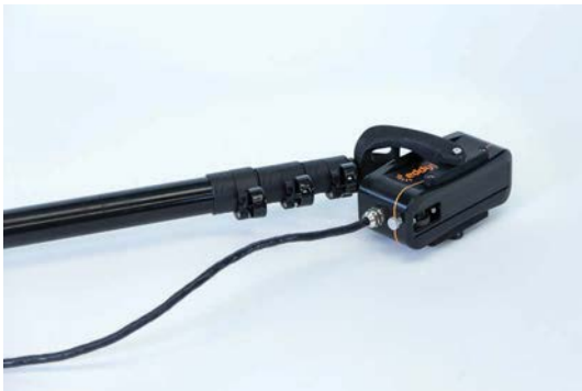
Figure C-4 Securing PEC probe to extension pole head
