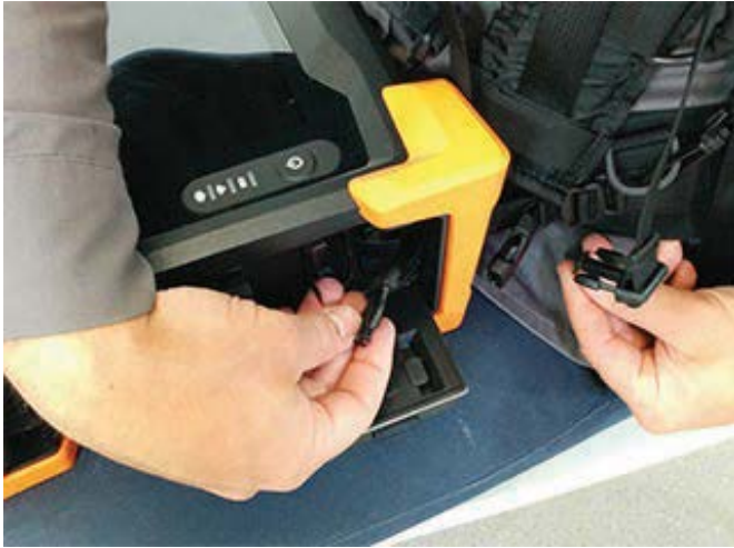
Figure B-12 Slipping male buckle through bumper
