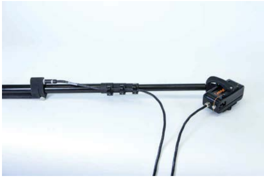
Figure C-6 Connecting PEC probe connector to extension pole remote control
